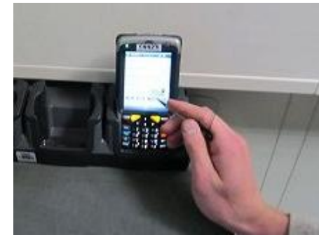
Data transfer to database and erp system over network connection by using wireless LAN or ethernet cradle (batch transfer)
