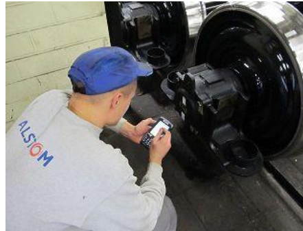
Data capture of wheelsets with handheld computer and software application from cosys running on mobile device
