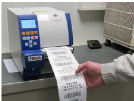
Printing wheelset label with stationary label printer (starting printjob from mobile device)
